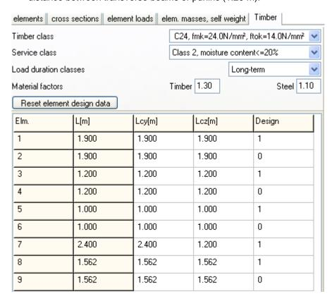
After you give all the data the timber design is performed according to Eurocode 5.
