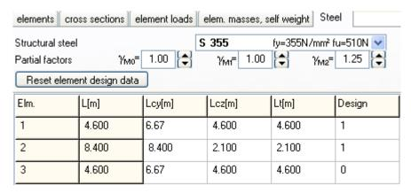
In order to define the buckling lengths of the columns for unbraced and braced frame according to Eurocode 3, use the extra tools of the program Design/Effective length of columns/Unraced members.
