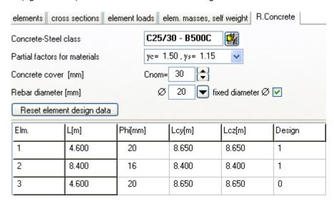
In order to define the buckling lengths of the columns for unbraced frame according to Eurocode 2 5.8.3.2, use the extra tools of the program Design/Effective length-Unraced members.
